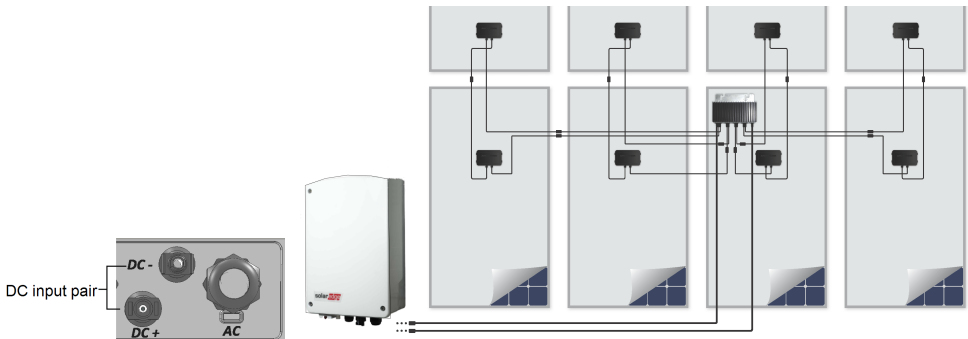
Figure 13: Inverter DC Connections
