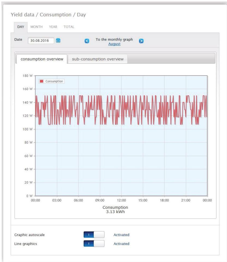
Fig.: Graph of daily consumption with meters connected and active line graphics
