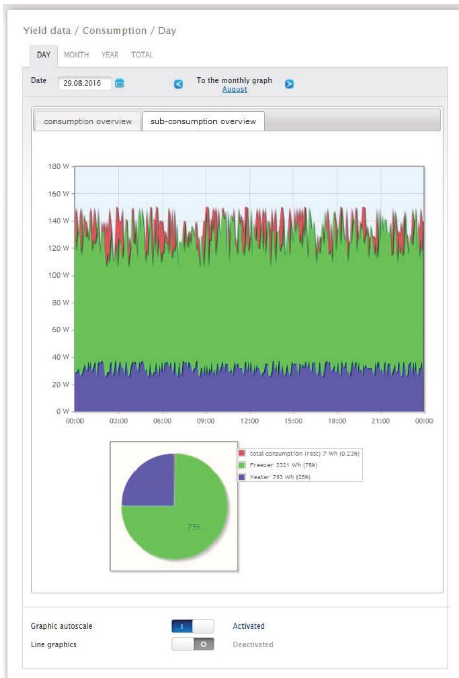
Fig.: Graph of daily consumption with connected appliances in the sub-consumer view
