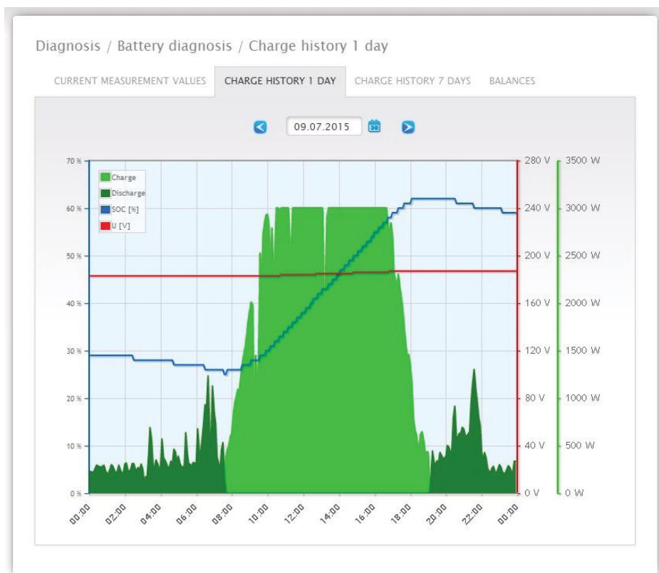
Fig.: Battery diagnosis - Charging History 1-Day
