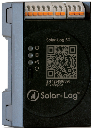
Fig.: Solar-Log 50 without extended snap-fit tabs
