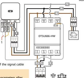
(1) Shield layer of the signal cable
