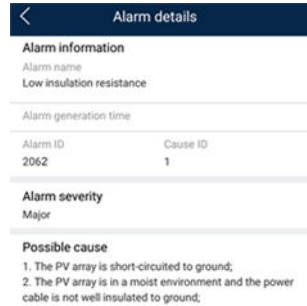
Figure E-1 Alarm details
