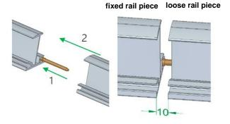
Push the connector into the secured rail piece up to half way into the screw channel, then push the lose rail piece with the screw channel onto the connector with a 10 mm gap between the rail ends, then attach the second rail piece.
