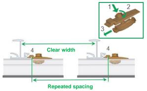
MV 9.2 Position of the cross rail connector IR
