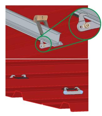
Position the trapezoidal sheet bracket with the aid of the mounting tool (1) on the insertion rail in the inclination of the raised bead with downward pressure.
