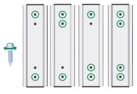
The static calculation in the system planning defines the number of fasteners required for mounting modules in landscape. For mounting modules in landscape the number of fasteners calculated with the design software is distributed on the raised bead as shown in the figure.
