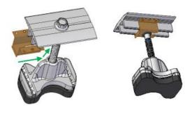
Push the contact latch on the sliding plate over the vertical webs of the middle clamp up to the screw.
