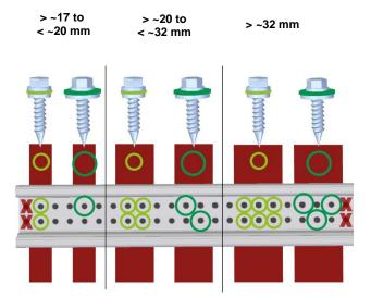
Mark the mounting position of the short profiles on the trapezoidal metal raised beads dependent on the module orientation – portrait or landscape, right-angled or on the raised bead – and the clamping areas specified by the module manufacturer. A gap of min. 10 mm must be maintained between the modules at the short frame side.
