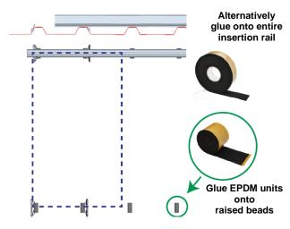
Mark the mounting axes of the insertion rails on the trapezoidal metal raised beads dependent on the module orientation - portrait or landscape.
