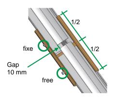
The number of fasteners is based on the static calculation with the fasteners shown.
