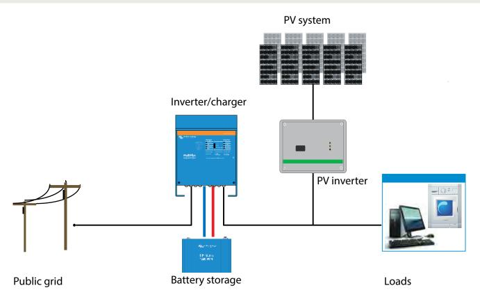
DC electrical power generated by the solar panels is converted to AC by a PV inverter connected to the AC output of an inverter/ charger.
