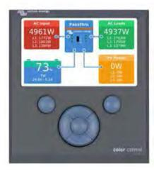
Color Control panel, showing a PV application
