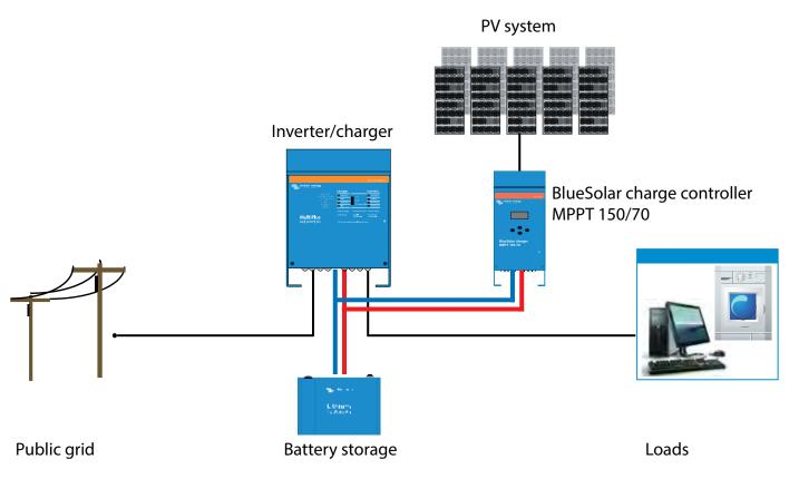
The BlueSolar MPPT charge controller uses solar power to charge the battery.
