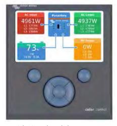
Color Control Panel, showing a PV application
