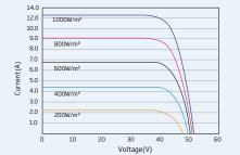
P-V CURVES OF PV MODULE(490W)
