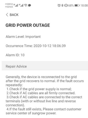
Figure 7-10 Detailed Fault Alarm Information
